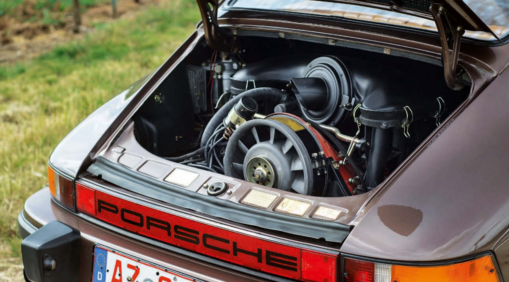
Above: The 2.7 MFI engine is what makes this 911 so special...
